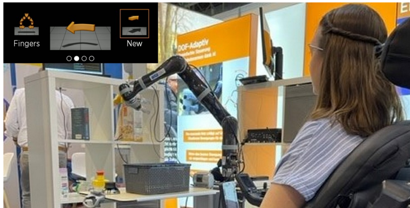
Figure 27: Study Apparatus at the Trade Fair of Study 3, illustrating the placement of user, table, and shelf, as well as the UI visualised on the smart glasses (top left). Reused from [VI] © 2024 IEEE
