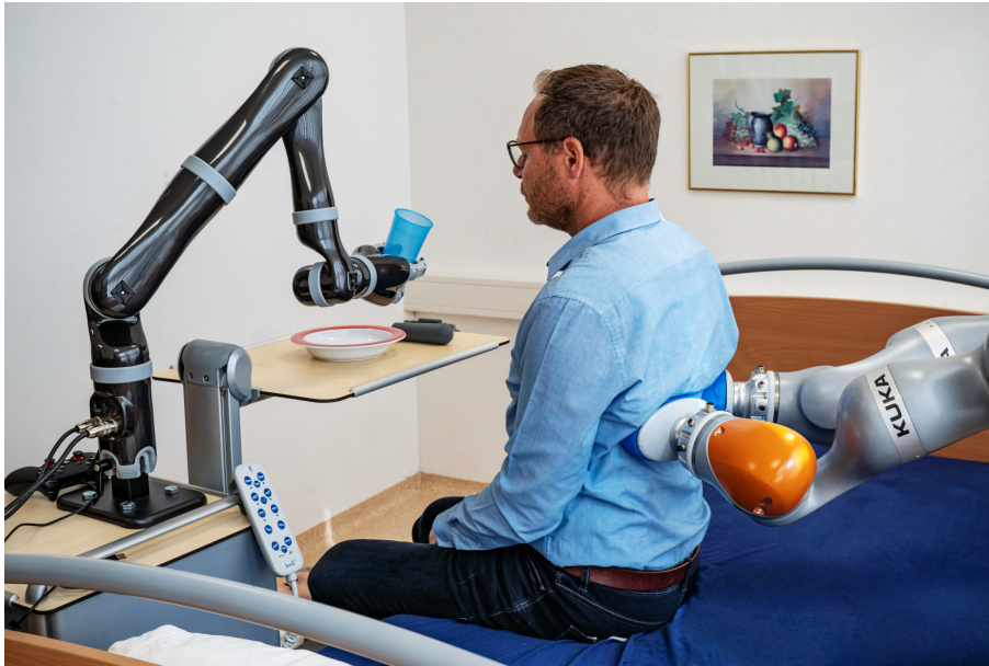
Figure 4: Demonstrator of the AdaMeKoR project with the patient-operated smaller robot on the left (main topic of this thesis) and the caregiver-assisting larger robot on the right. Courtesy of DFKI
