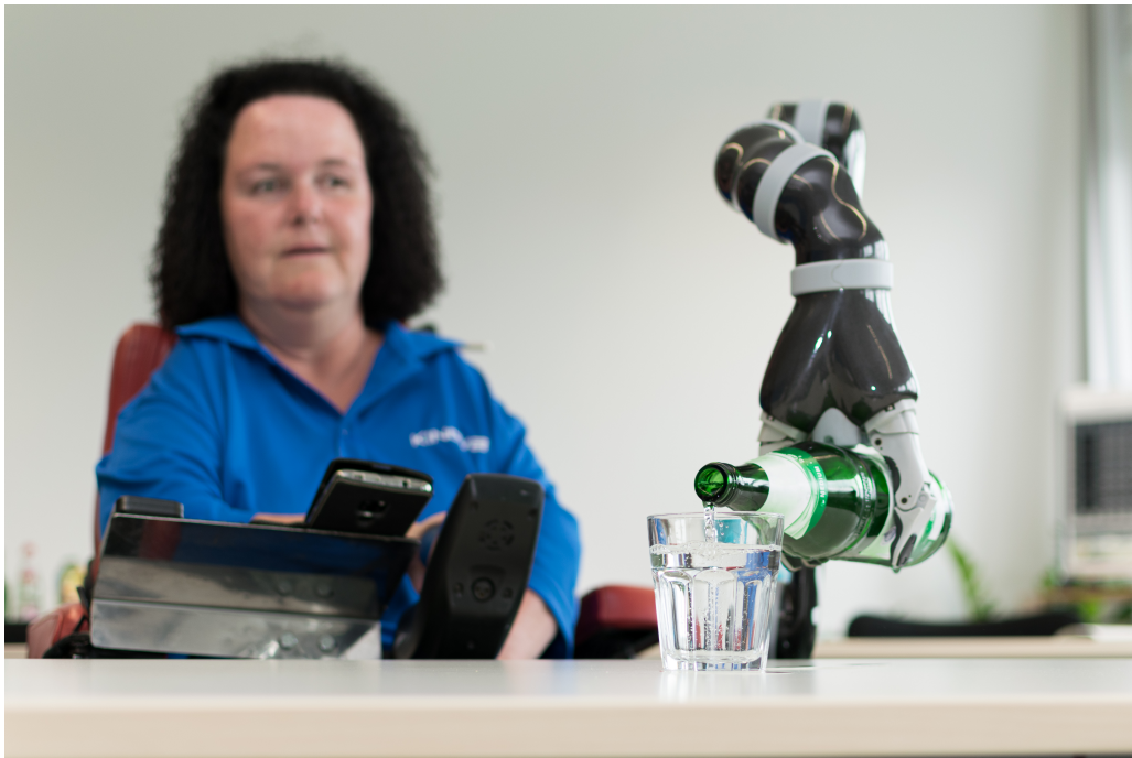
Figure 1: The Kinova Jaco Assistive Robot Arm as WMRA. Courtesy of Kevin Rupp | Frankfurt UAS
