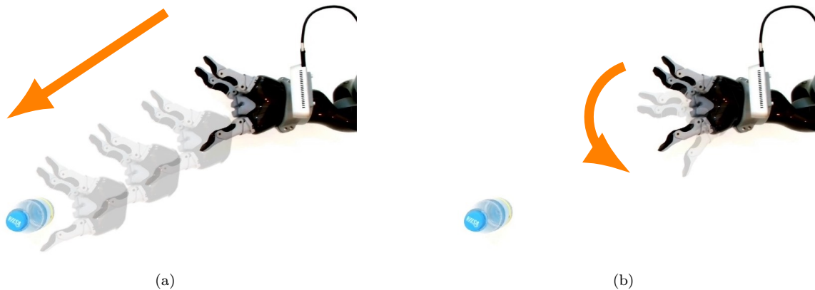
Figure 24: Two Classic Behaviours of (a) Approaching an Object and (b) Rotating towards it. Represented top down using a Jaco robot with ghosts and arrows to show motion. Adapted from [V]
