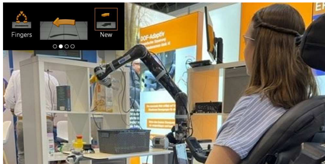
Fig. 1: Study apparatus at the trade fair, illustrating the placement of user, table, and shelf, as well as the UI visualized on the smart glasses (top left)
