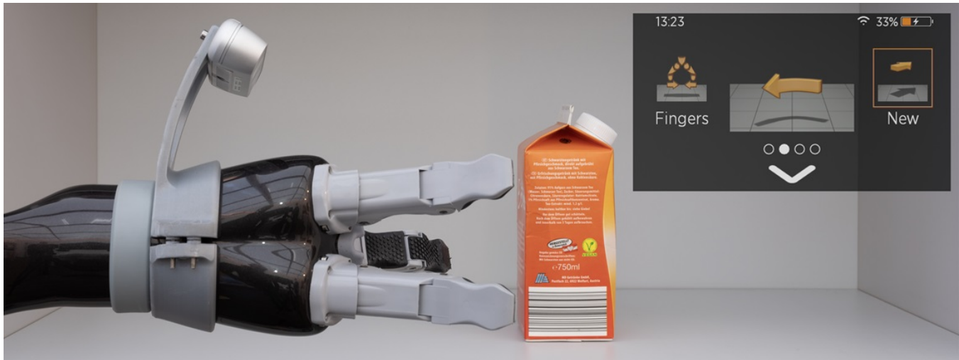
Figure 1: User Perspective of the Adaptive DoF Control, including a robot arm with wrist-mounted camera (left) and the user interface as shown on the smart glasses (right)
