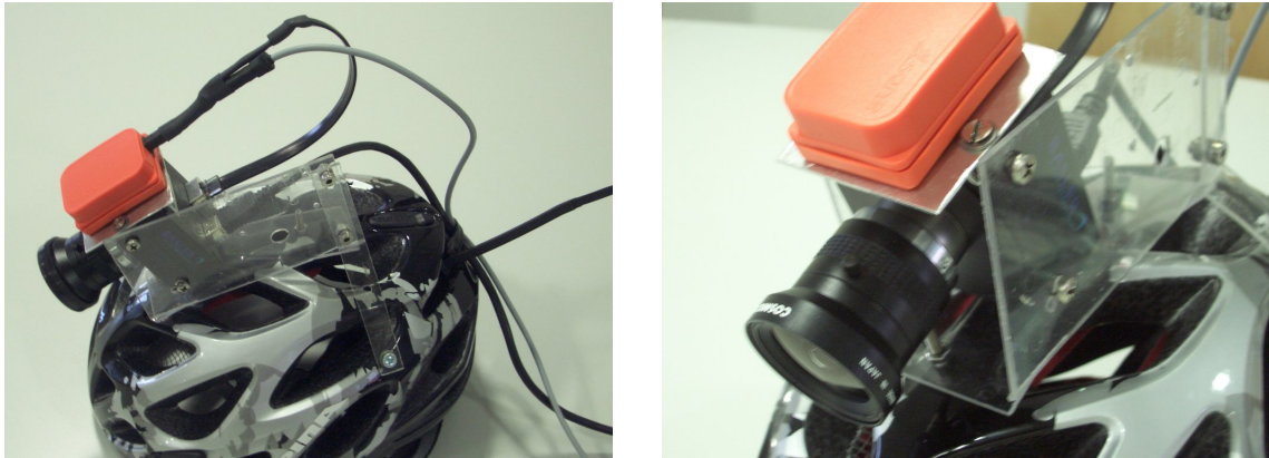
Figure 5.1: Used sensor setup for the experiments. (Left) The sensor setup viewed from the side. The photograph shows how the inertial sensor is mounted on top of the camera, the connection cable of each sensor and the synchronization cable between both sensors. (Right) The sensor setup shown from the front. The camera is mounted inclined onto the helmet so the view of the person wearing the helmet matches the view of the camera.
