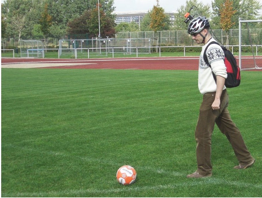
Figure 1.1: Camera-inertial sensor attached to a helmet worn by a human. This setup was used during the experiments.
