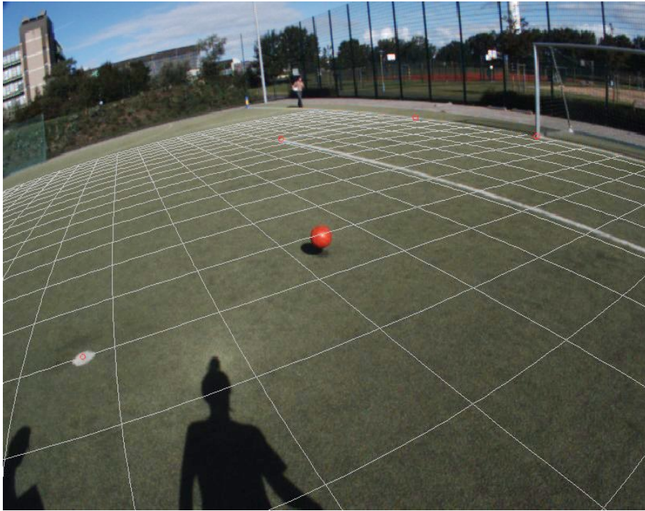
Figure 5.3: Grid overlay created by a homography between points on the image plane and points on the field plane. The four points chosen for the homography estimation are marked by red circles. The space between the lines is 1 m . It can be seen (especially near the front line of the goalkeeper's area), how well the grid resembles the actual plane on the field. The image here shows a ball right after it bounced off the ground. The position of the raised dust is used to determine the actual bouncing point of the ball on the field.
