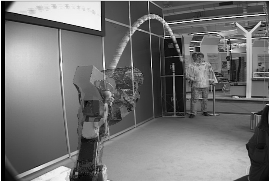
Figure 1.3: Video sequence overlay of a successful catch by the robotic ball-catcher showing the trajectory of the thrown ball. Image courtesy of [7].
